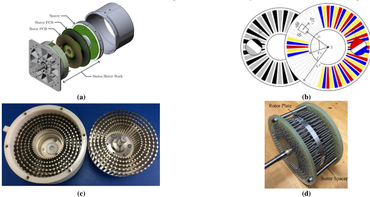
Figure 1: Proposed structures for electrostatic motors a), b) axial motor and its components, c) , d) peg style and its component
