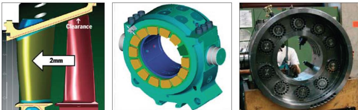
Figure 8. Hydraulic clearance optimisation (HCO). From left to right: movement of rotor; modified bearing for HCO upgrade of SGT5-2000E/V94.2; modified bearing for HCO upgrade of SGT5-4000F/V94.3A
